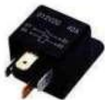
4P Relay, with Bracket 12V 40Amps/24V 40Amps SPST, NO Type
