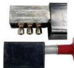
2 Speed Axle Switch 12VDC, 30Amps 3 Snap-in Terminals, Die-Casting Body protected with Rubber Cover. Use with Eaton Two-Speed Rear Axle. Replace: Eaton 32861 Diamond T/Reo 9935-H, 319305 Dodge 1390517 Ford 8QH-4078, SW-1535 GMC 2274282, IHC 79348-R91 Mack IMR-2101, White 716913
