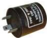
263 Flasher 3P 12V Max 20Amps 2-10 Lamps Np-Polarized.
