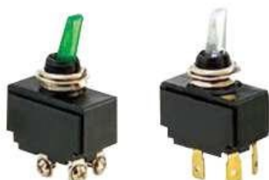
Illuminated Toggle Switch (Blub) Single Pole/Double Pole 12VDC 10Amps With Green Lever or White Lever. Meet IP54
