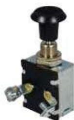
Universal Headlight Switch 12VDC, 15Amps. Switch is ON when pulled out. 2 Position - OFF/ON, 7/16" Diameter.
