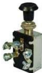
Universal Headlight Switch 12VDC, 15Amps. Switch is ON when pulled out. 5 Screw Terminals. 3 Position - OFF/ON/ON, 7/16" Diameter.
